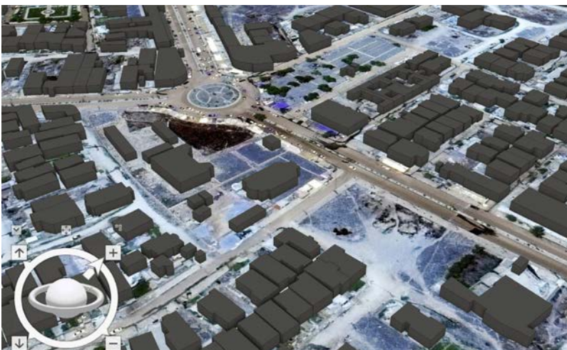
A MAG pilot project implemented in Sinjar with funding from the Ministry of Foreign Affairs of the Netherlands, employed digital elevation software to derive and represent buildings in a three-dimensional model.
